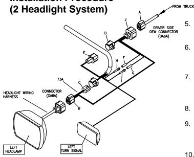
Figure 1. Driver Side Single Connections
