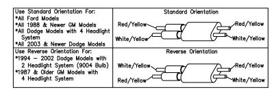
Figure 3. Vehicle Option Connector
